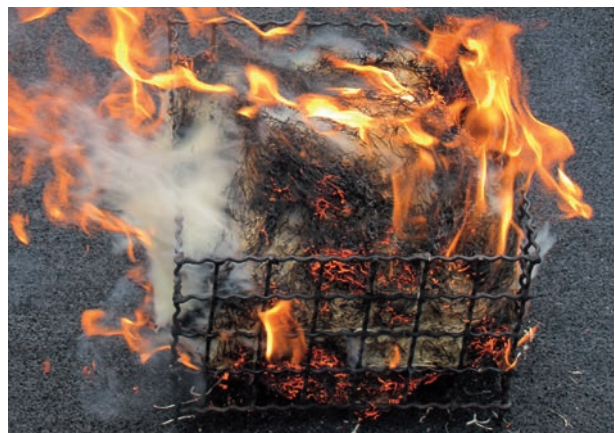
The diameter of the burn mark is only insignificantly larger than the fire basket. The fire did not penetrate the building protection sheet.
