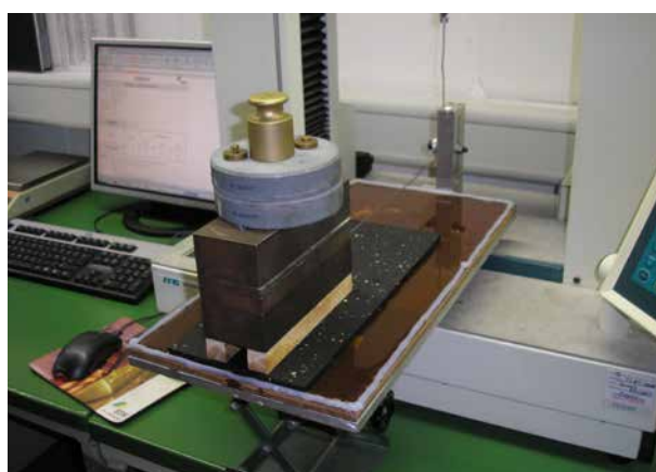
The sliding friction coefficient of the Regupol® Anti-Slip Mats , with the respective material combinations, will be determined in our own laboratory (above and below).
